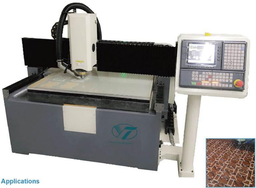
HD1100 pertinax machine is mainly for cutting the pertinax in Sandwich die industry,
